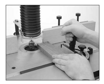
Figure 23. Using the miter gauge.
